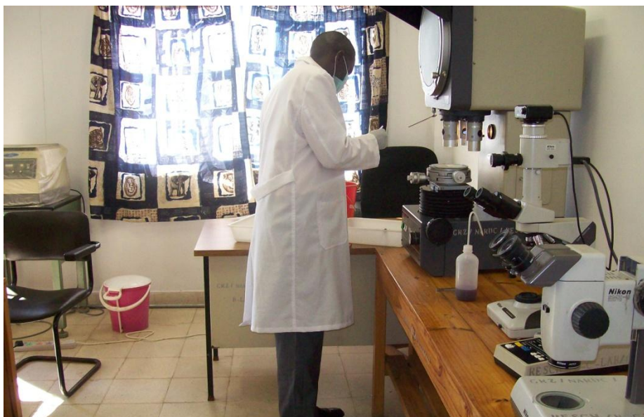
Oreochromis andersonii masculinisation verification on a profile microscope
