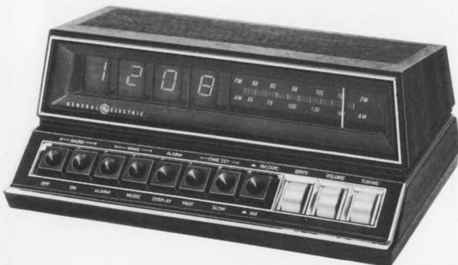
This GE clock radio has an 822-transistor LSI chip. The time is displayed from 1:00 to 12:59 in one-minute steps, while the alarm is set in increments of 10 minutes.
