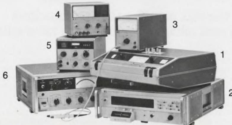
No. 1: 4342A Q Meter. No. 2: 4270A Automatic Capacitance Bridge. No. 3: 4328A Milliohmmer. No. 4: 4329A High Resistance Meter. No. 5: 4260A Universal Bridge. No. 6: 4470A Transistor Noise Analyzer.
