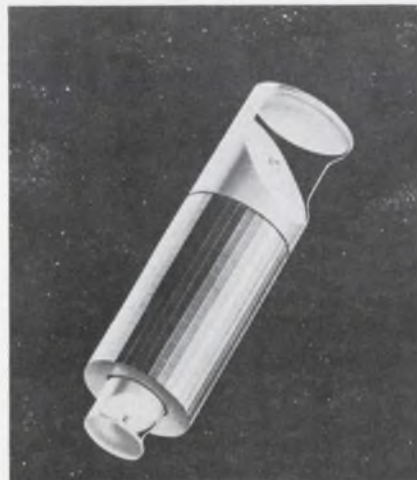
AT&T proposal for a mixed earth-space communication system would have four satellites in operation by 1980. The satellite at right would use both pulse-code and frequency-modulation techniques and be capable of providing 12 TV channels and more than 30,000 duplex voice circuits.
