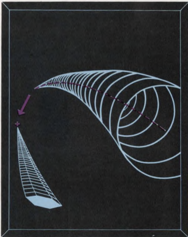
2. Manual rendezvous is accomplished through the use of a visual display. If any course correction is required during rendezvous, this is indicated by the error vector (arrow).
