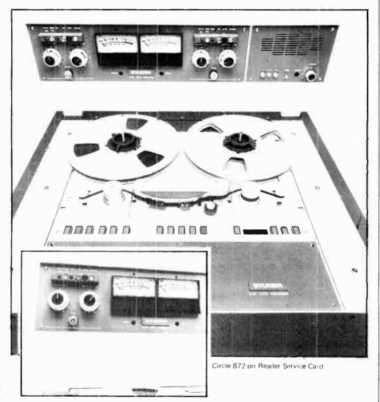
The right side of the penthouse contains a five by three-inch elliptical speaker with a panel containing a volume control, phones socket, repro/input select and to select channel 1, 2, 1+2 input to the speaker. There is ample volume from this speaker for editing and other machine local operations but I found it very easy to leave it on and not realize that I could still hear it while sitting in front of the studio monitors and so color
