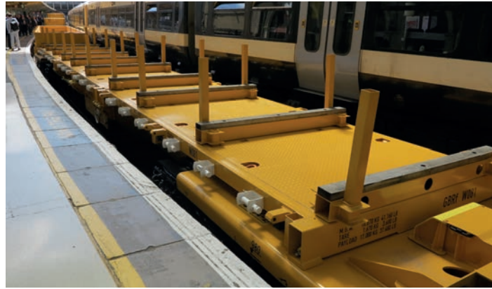
On display at London Victoria were FEA-W flat wagons with different superstructure modules, plus MLA and JNA box wagons for ballast and aggregates.
