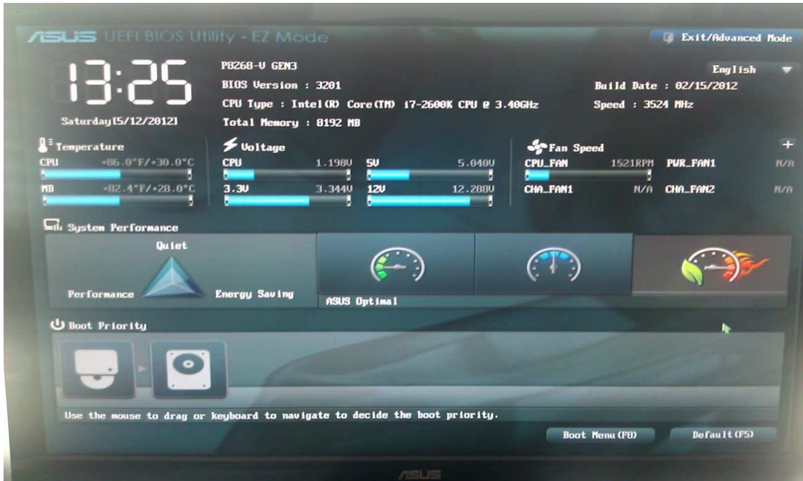
FIGURE 4. Asus p8z68-v/gen3 motherboard bios main screen in asus ez mode. Power settings can be changed and forced from BIOS to work under Windows operating system.
