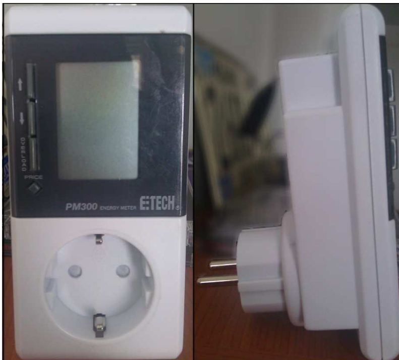
FIGURE 2. Etech pm300 energy meter. Front and side figure of used ETECH PM300 energy meter
