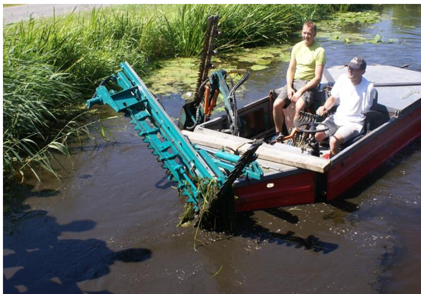
Figure 8.1: A weed cutting boat with mowing gear (Photo: R. Pot).
