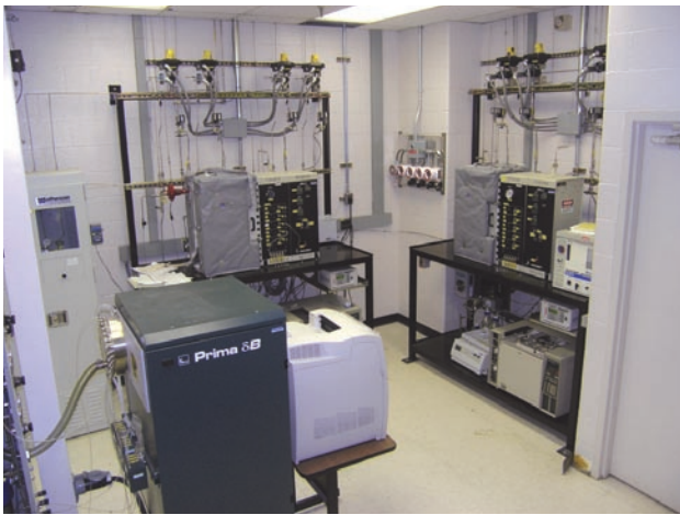
FIGURE 2. Fuel Processing Laboratory with Twin-performance Reactors, Online Mass Spectrometer and GCs
