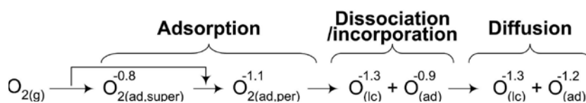
FIGURE 3. A Stepwise Reaction Mechanism of Oxygen Reduction on a Defective LMO Surface
