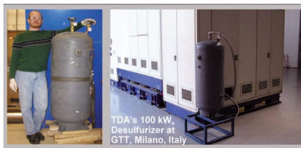
FIGURE 1. Pictures of the Two 100 kW TDA Desulfurizers
