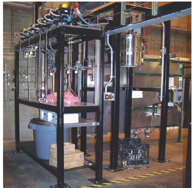
FIGURE 3. Fuel Processing Unit: A Test Stand Capable of Testing 10-28 kW Reformers
