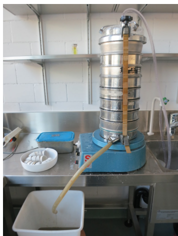
(a) Set up for the wet sieving of the sediments
