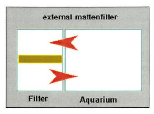
Other aquarists have moved the Mattenfilter out of the tank, into a second tank, i.e. a sump. If the balance between the size of the combined tanks, the flow rate and amount of water filtered is preserved, there really is no argument against this sort of setup. With some DIY it could even be possible to hide a sump setup underneath the tank.
