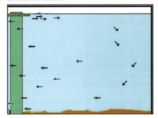
Drawing 2 shows a setup powered by an air pump. The air lift sits behind the mat. The exit tube sits in a carved out slit at the top of the mat and sticks out 5 cm to ensure that small fish will not crawl through. Some species seem to like this. These animals almost seem hypnotized by the current and are drawn into it.
