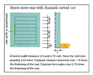
My smallest tanks are no bigger than 5 liters. These are photo tanks. I have used a construction there whereby the channels for transporting the water are carved out of the back of the foam, rather than leaving 2 cm between mat and glass.
