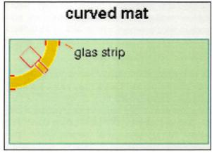
The radius should be calculated to have the required surface. The actual curve should not be too small, because the inside of the mat is compressed somewhat and will slow down the water flow a little. How far you can go depends on the actual type of foam used and its thickness.
