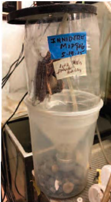
2-liter coke bottles (with bottom removed) corked and inverted into, (left) a repurposed quart sized clear plastic deli-ware container; and, (right), a four-inch PVC fitting.
