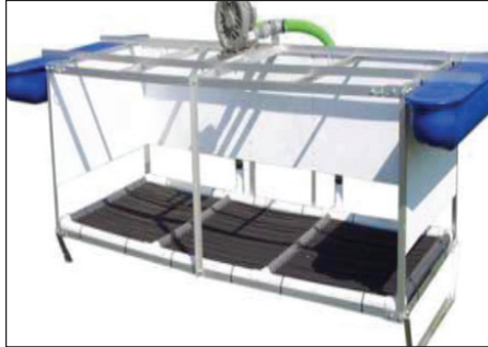
Air tubes with 0.1-2.2 m 3 air/meter/hour, efficiency is diameter and depth dependent
