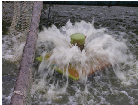
Left: In-pond RAS – an intensive unit aerated with airlift. Center: An aerator set at the side of a cage. Left: The schematic operation of an air lift (1. Blower. 2. Continuous suction of water and 3. Continuous flow of water).
