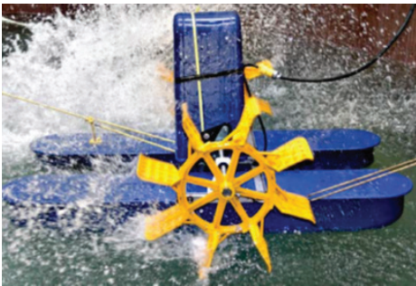
Surface, paddlewheel aerator with an efficiency of: SAE: 1.2-2.9 kg O 2 /kWh
