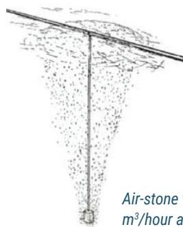
Spray aerator with an efficiency of: SAE: 0.06-0.17 kg O 2 /kWh
