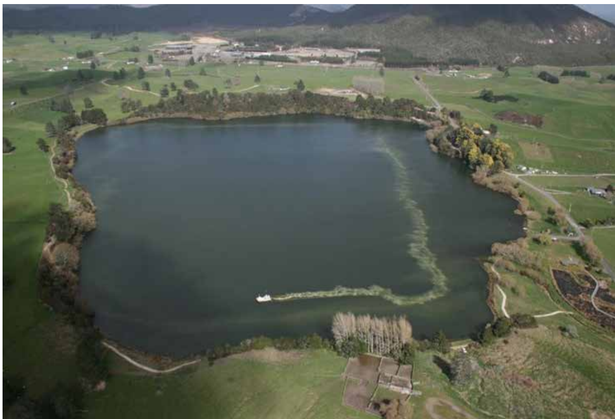
Figure 5.8 Trial of geoengineering in 2009 using a chemical amendment (e.g. modified zeolites and bentonites) to reduce phosphorus concentrations in the water column in Lake Okaro, New Zealand. Photograph courtesy of Andy Bruere, Bay of Plenty Regional Council, New Zealand.
