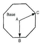
A = Axis of Rotation AB = Minimum Radius AC = Maximum Radius
