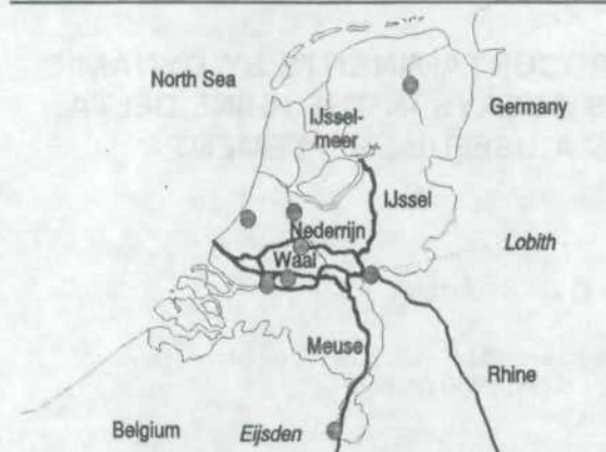
Figure 32. The Rhine delta with surface- and drinking water control stations equipped with a early warning fish monitor. In addition, waterflea monitors are located at Lobith and Eijsden.
