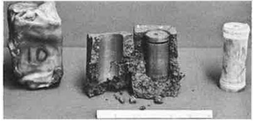
Figure 2. Compacted soil piece in wax (left), cylindrical split mold with soil core in it (center), and trimmed sample in a rubber membrane with Lucite disks on top and bottom (right).
