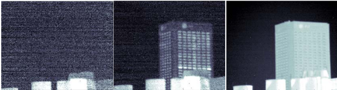
Figure 352. IR image at 1076\text{ cm}^{-1} of the scene on January 18, 2011, visibility 2 miles (left panel). IR image at 1076\text{ cm}^{-1} of the scene on January 20, 2011, visibility 6 miles (middle panel). IR image at 1076\text{ cm}^{-1} of the scene on January 28, 2011, visibility 10 miles (right panel).
