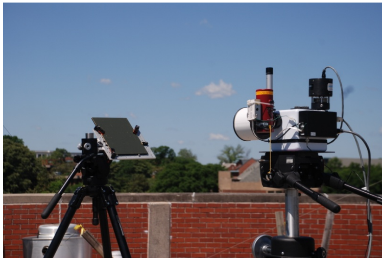
Figure 74. The D&P test setup for the zenith sky measurements.
