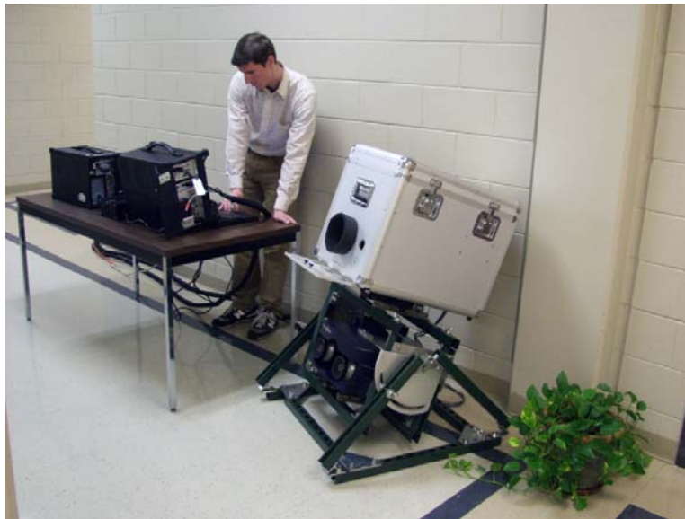
Figure 182. The final mount for the D&P and Hyper-Cam.
