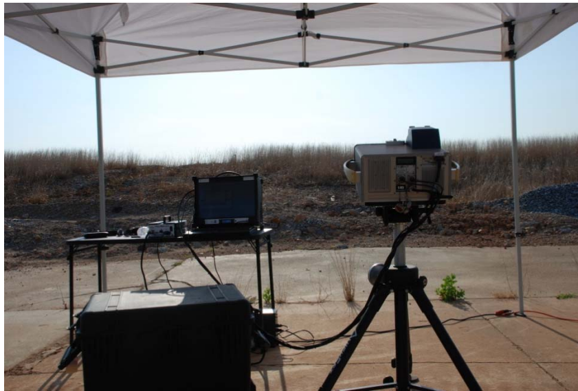
Fig. 2. The Hyper-Cam set up to image oncoming aircraft.
