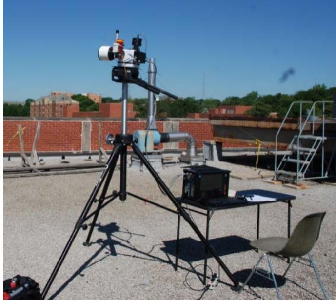
Figure 73. The D&P test setup for the five degree elevation sky measurements.
