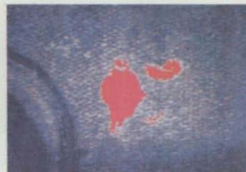
Aluminum Honeycomb Panel inspected with shearography showing cells and unbonds.
