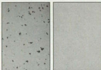
Photomicrograph shows microshrinkage in as-cast condition A356 aluminum. Magnification: 3x
