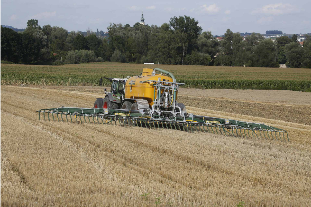
Figure 4.8 Farmer applying phosphorus-rich slurry to a field using a trailing hose. Trailing hose and slurry injection techniques offer the potential to reduce dissolved phosphorus concentrations in runoff during the period immediately after slurry application.
