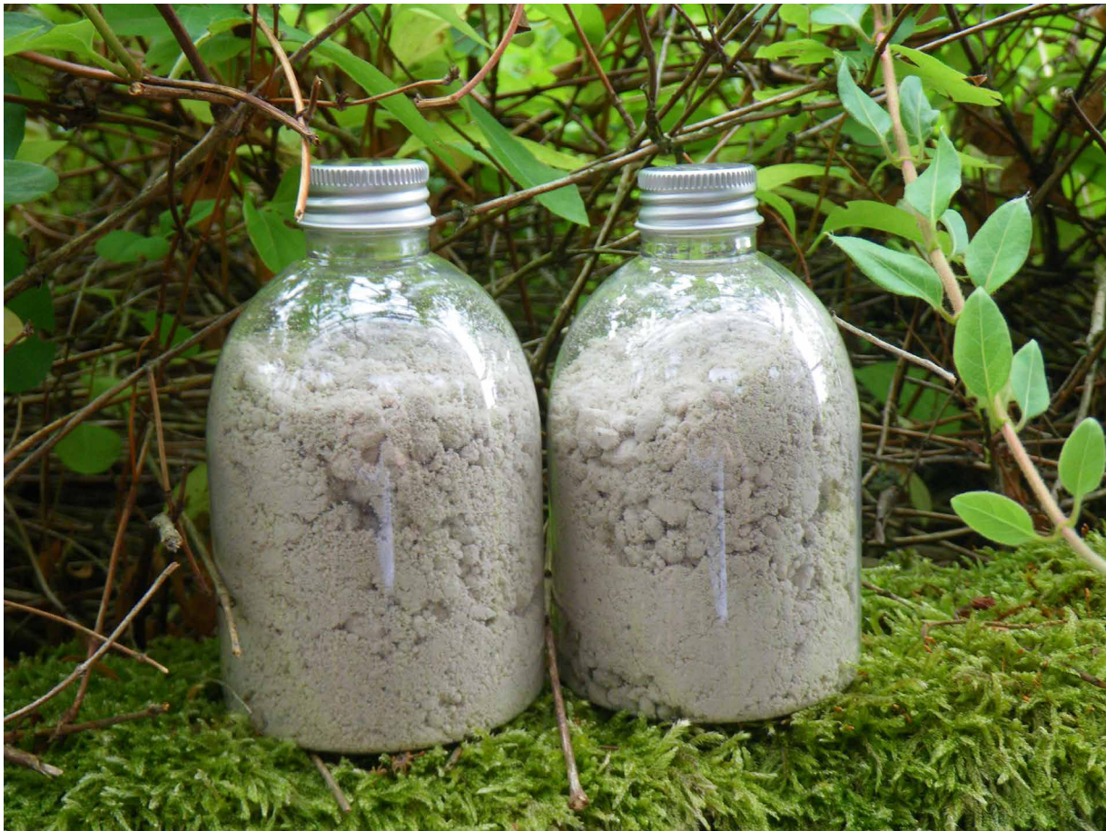
Figure 7.3 Phosphorus recovered from wastewaters in the form of struvite produced from a Huber SE precipitation reactor. Photograph courtesy of The Sustainable Sanitation Alliance (SuSanA).
