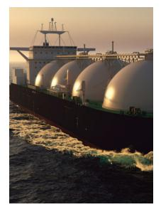
Cryogenic applications such as LNG storage and shipping use steel containing 9% nickel.
