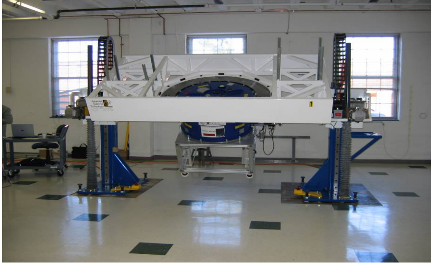
Figure 4-5. NRAO FEIC Tilt Table with cryostat attached.
