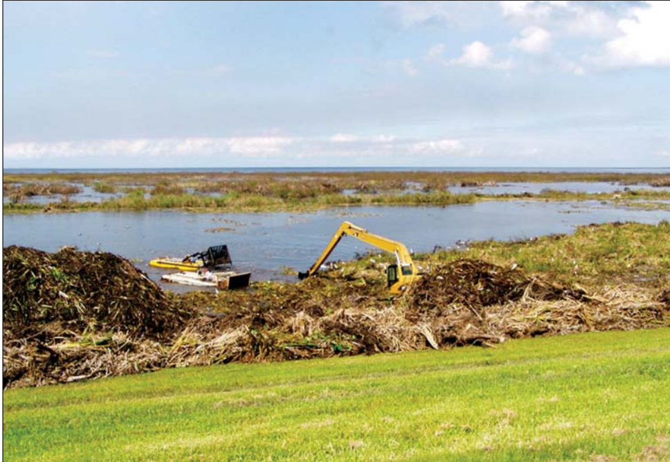
Figure 24. Mechanical removal by operating a harvester with removal belt (top) and by pushing weeds on shore for harvesting with a track hoe (bottom). Photographs by Jeff Schardt (top photo) and unknown (bottom photo), UF/IFAS Center for Aquatic and Invasive Plants.
