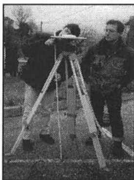
Picture 3: Student measuring the slope instruments height of the GPS antenna.
