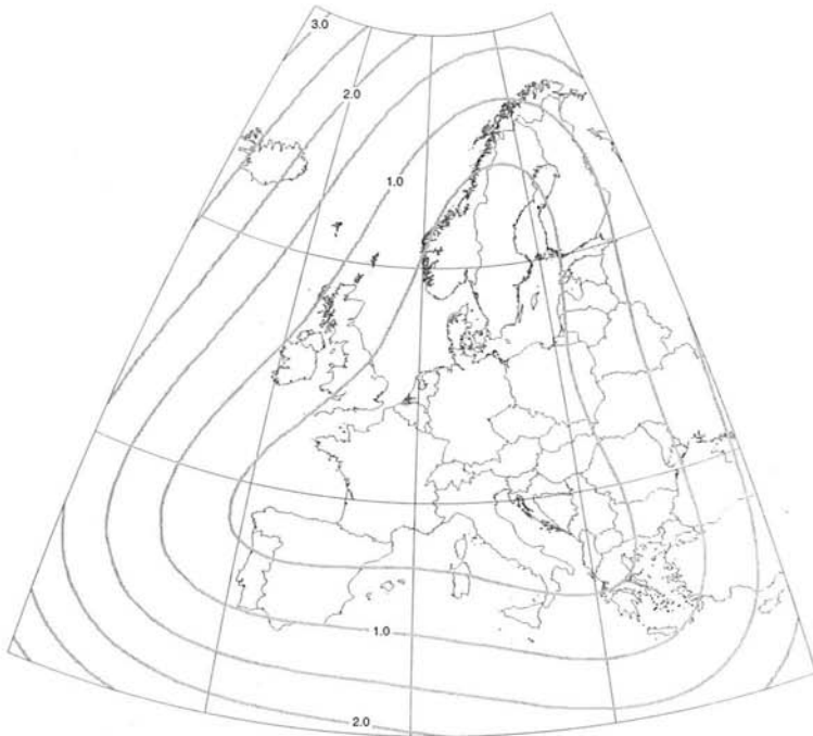
Figure 3. Low-error equal-area projection for the European Union with lines of constant maximum scale error (%)
