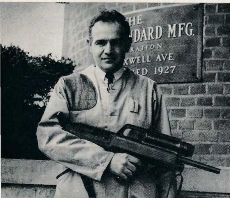
High Standard's Model Ten police weapon is a radical departure from a shotgun's normal lines, despite its adaption from the Supermatic. Sold to police units exclusively, it fires magnum or express loads only.
