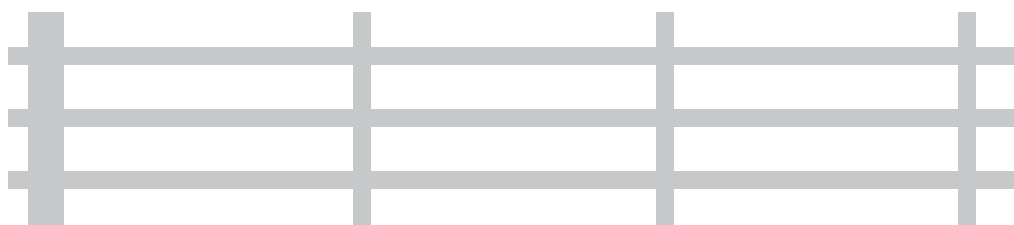
MAX-FLOW 68% OPEN SLOTS 1/4" X 1-1/2", IN ROWS ACROSS WIDTH OF SHEET. VERTICAL BARS 3/32" WIDE, WITH EVERY THIRD BAR 3/16"
