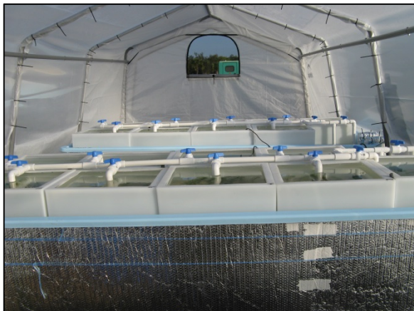
Figure 2. Experimental tanks were set up in four fiberglass troughs, one for each one of four temperatures.
