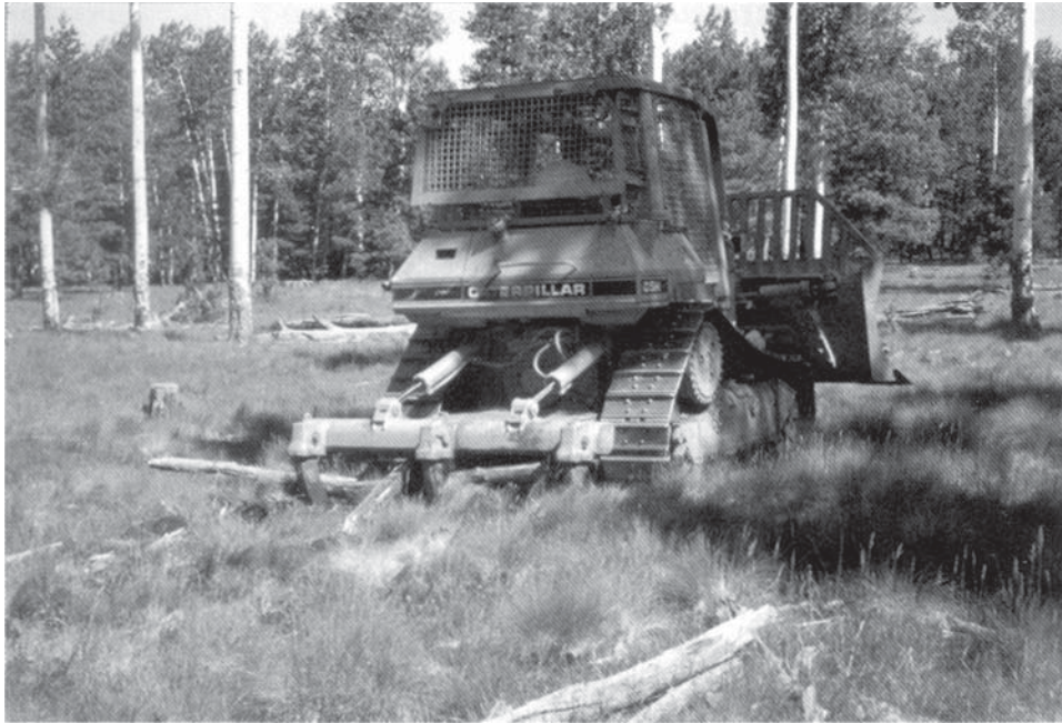
Figure 6 —Severing lateral aspen roots using a dozer-mounted ripper, Coconino NF, Arizona.
