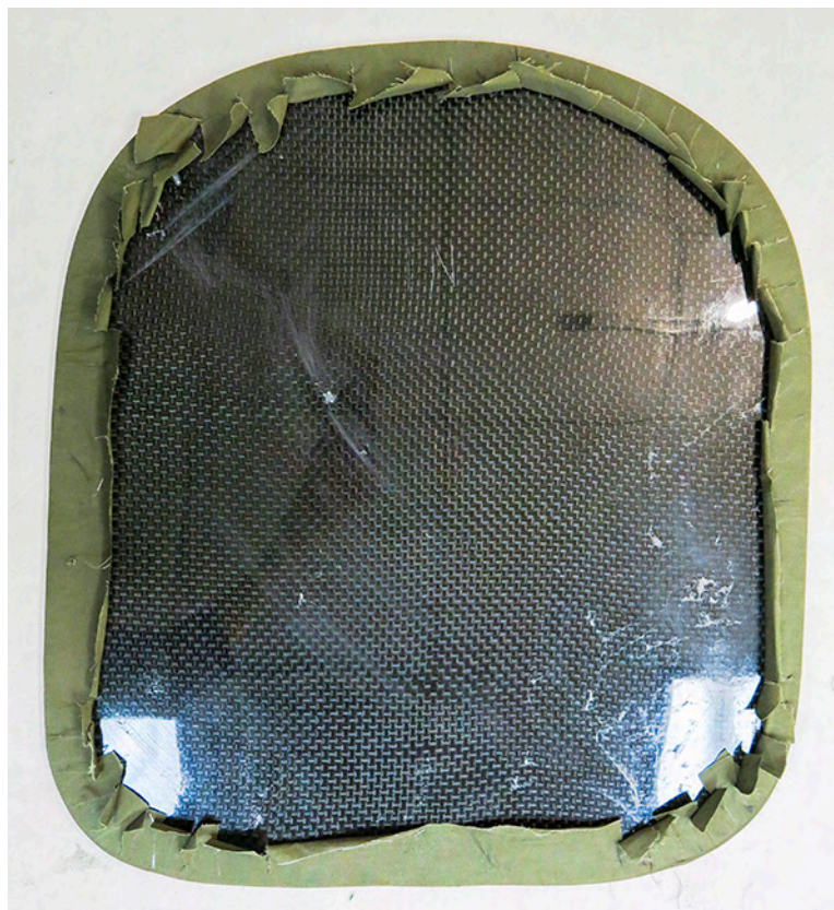
Fig. 4. Inner back unit: The CF plate is covered with green cotton broadcloth using Beva 371 thick film to adhere it to the back around the edges.
