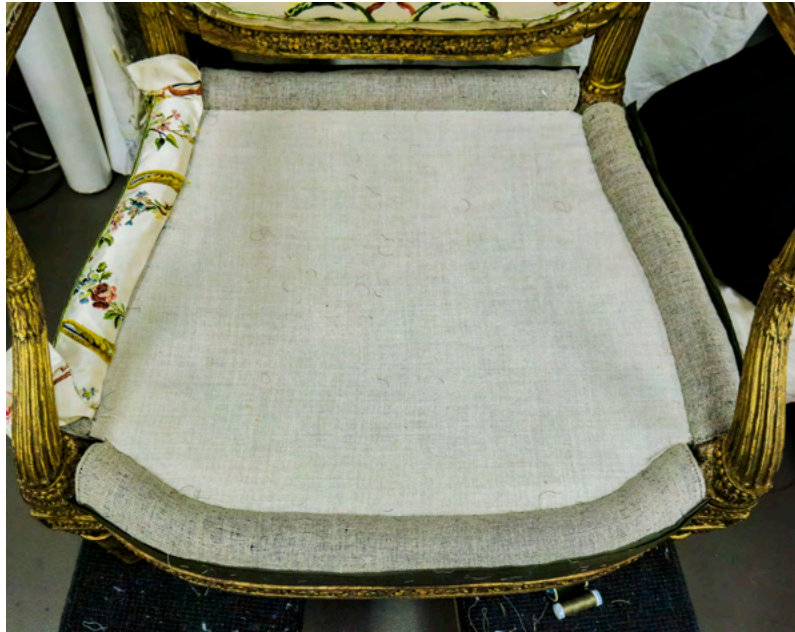
Fig. 12. Conservation seat: The linen deck is sewn to the inside of the edge rolls and the showcovers are stitched on.
