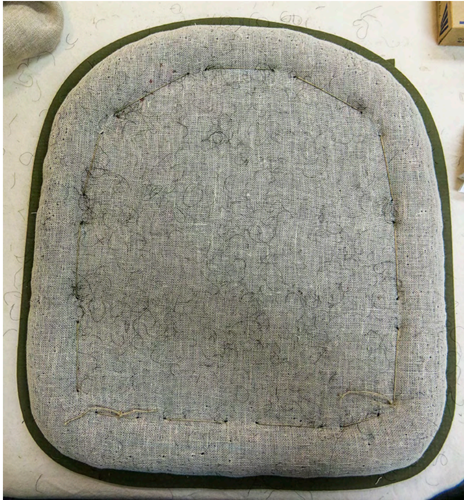
Fig. 6. Inner back unit: The edge rolls are made using linen stitched down to the CF, then filled with horsehair and stapled to the outside edges of the wood frame.
