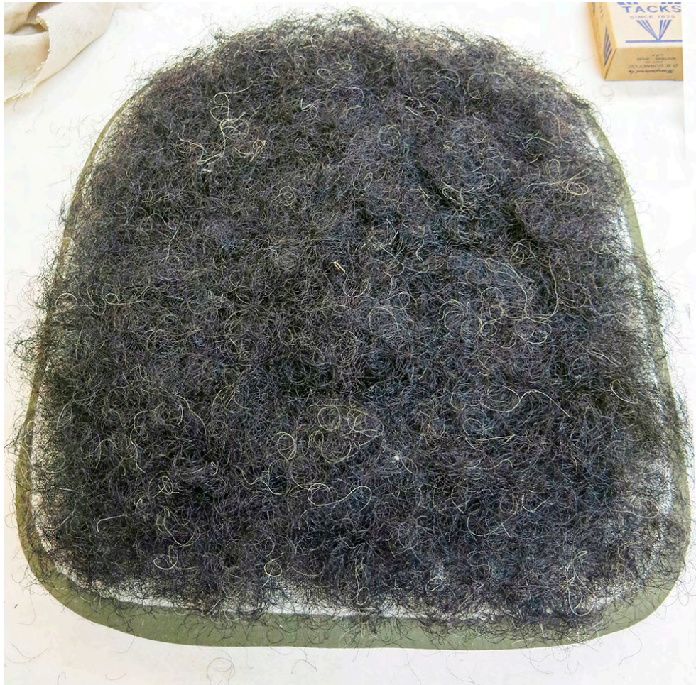
Fig. 7. Inner back unit: The well is filled with horsehair and then compressed and covered with high-count ticking.
