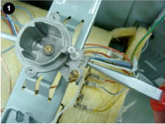
1.Remove spark plug clip.
