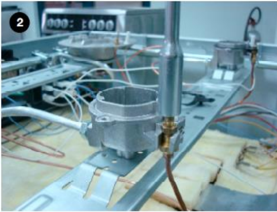
2.Unplug the thermocouple.
