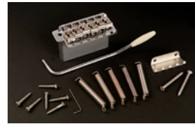
Gotoh Master Relic Collection tremolo, pitch 11,3 mm, steel block, steel sheet metal saddles with USA thread screws, 6 pivot points
