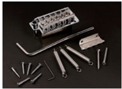
Gotoh tremolo, pitch 10,8 mm, steel block, steel sheet metal saddles, 6 pivot points
