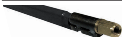
Boston truss rod 18320 TRO-600-L bar model 6mm, 7mm hexanut "G-style", UNF-10-32 thread, 600mm., single action
