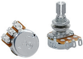
Alpha small 25K audio potentiometer 42007 ALPS25-A55 16mm. 10mm. bushing, M7x0,75 thread
