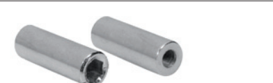
Boston truss rod nut 30283 TRN-20 allen nut, allen key size 4mm, UNF-10-32 thread
