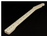
Allparts neck for Telecaster® 47610 TMOFAT chunky, maple fretboard, 9,5" radius, 21 tall frets, sanded/unfinished
