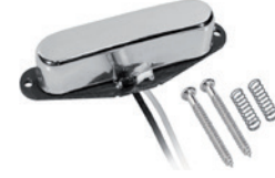
Boston Vintage single coil pickup, Alnico 5 rods, black fibre bobbin, waxed formvar wire, 7.5K, neck
