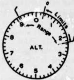
FIGURE 8.1—Sample score sheet used for the range and limit methods of measuring altitude in the steep turn. (Reduced to \frac{1}{2} size used.)
