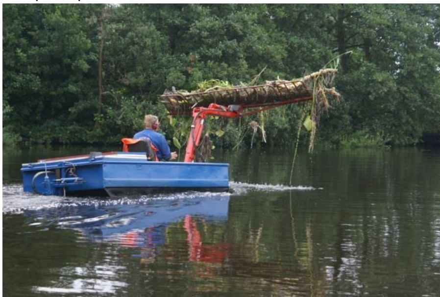
Figure 8.2: A harvesting boat with a hydraulically controlled rack for collecting floating plants, in use in the Netherlands (Photo: R. Pot).
