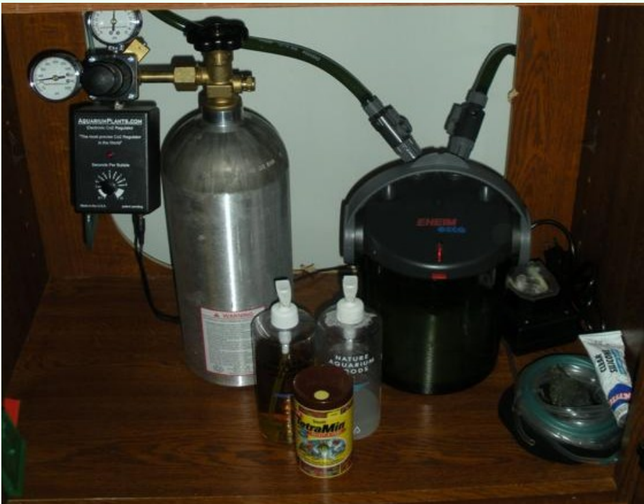
DIY CO 2 setup was quickly replaced with a pressurized CO 2 unit to ensure consistent gas injection into the water column.
