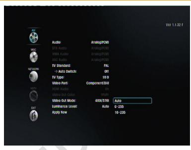
New is the "Luminance" mode where you can select between the usual 0-255 (PC Black White levels), 16 – 234 (Video Black White levels) and an Auto Mode where the TVIX will be following up on information that the display provides to TVIX through HDMI
