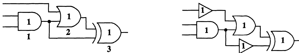
Figure 13. Buffer insertion for path balancing.
