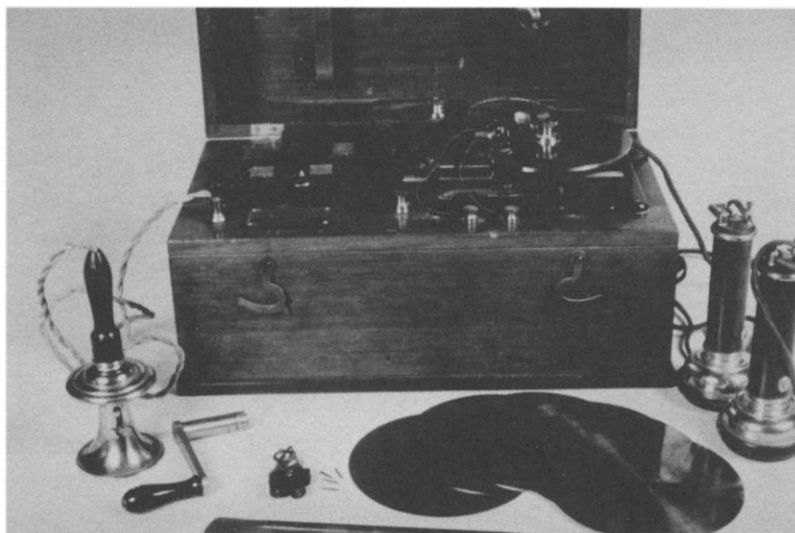
Danish disk type telegraphophone, built in the period 1905-09 when E. Hytten was director of Dansk Telegrafonfabrik in Copenhagen. The disk is 0.5 mm thick and 130 mm wide steel plate, rotating by means of a clockwork drive. The velocity of the disk relative to the reading/writing head is 0,5 m/s. (Photograph courtesy of the Danish Museum of Science and Technology.)
